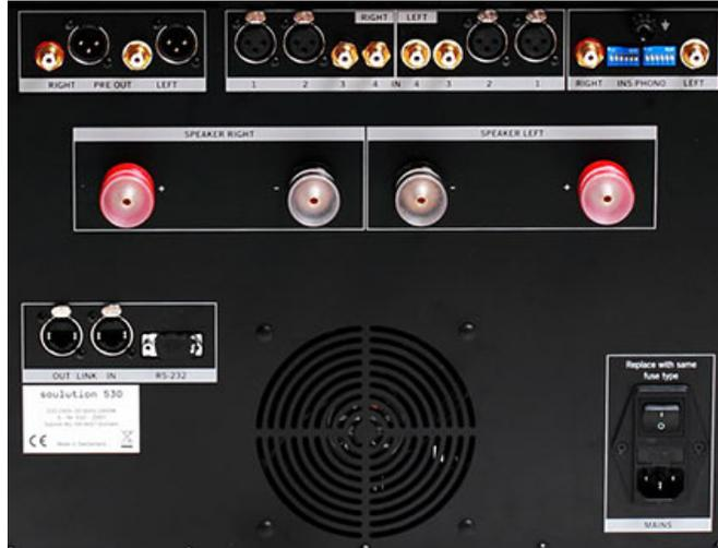
The 530 has dimensions of 350 x 448 x 442 (HxWxD in mm), weighs around 90 pounds and delivers up to 125 W at 8 Ohm, 250 W at 4 Ohms and 500 W at 2 Ohm, thus acting as an ideal current source. The amplifier's finish is fantastic – no bolts in sight, perfect components fit. The whole unit is an extremely rigid, vibration-resistant block that will likely outlive more than one owner. External design may not appeal to everyone but it is timeless. Fashions come and go, and simplicity remains.
