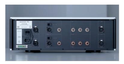
The line stage soulution 721 provides three unbalanced (WBT Nextgen Cinch) and one balanced XLR-input. Balanced and unbalanced outputs connectors are available.
