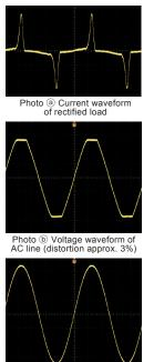
Photo © PS-530 output waveform (distortion approx. 0.06%)
