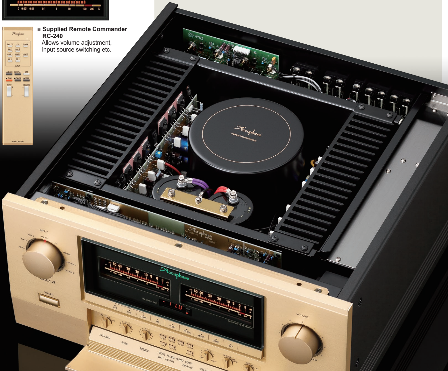
Speaker terminals connected directly to protection circuitry
